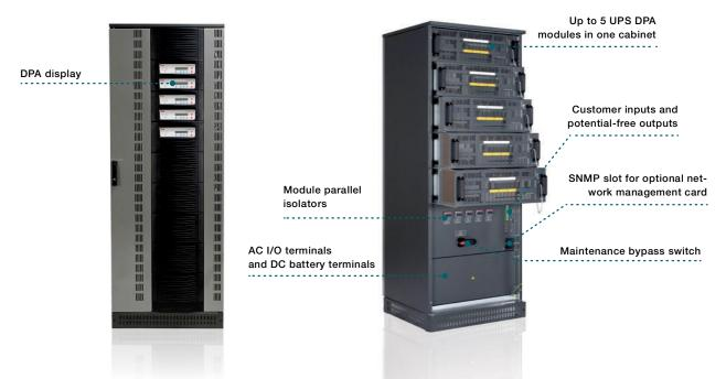
The Conceptpower DPA is a true double conversion modular UPS designed for medium-sized critical applications. The Conceptpower DPA's modular architecture provides very flexible power configuration based on 30/40/50 kVA modules that can be added as power requirements grow—
